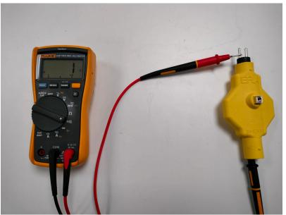
4. If the functionality of the sheriff is still in doubt after the first 3 steps (light doesn't function normally etc.) Please check the continuity of the sheriff unit. Continuity has to be measured between the large pin - large socket and small pin - small socket. Multimeter continuity function can be used. Both sides of the sheriff unit must have continuity for the unit to function properly.
