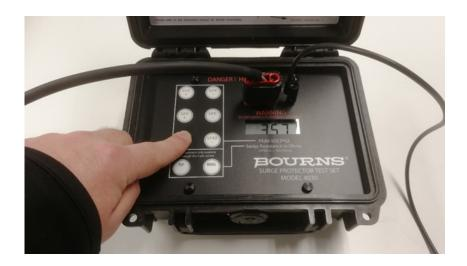
3. If the readings are inside the tolerance (350  $\pm$  50). Components inside the sheriff are fully functional.
