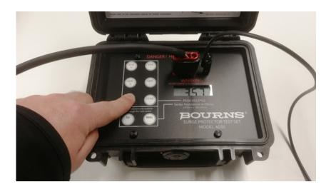
3. If the readings are inside the tolerance (350  $\pm$  50). Sheriff is fully functional.
