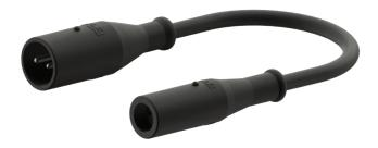
Frangible KDC7 connector is designed with break-away point and protected with a special sleeve. Upon an impact, connector breaks safely and does not cause additional hazard, like ignition of kerosin. KDC7 connectors are fully compliant with ICAO Aerodrome Design Manual Part 6, frangibility requirements.
